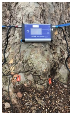
Tree works and PiCUS scan at Plane
